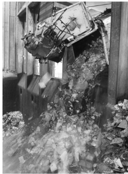
Figure 4: Waste is being brought to the waste cleft of the waste combustion plant of Kyläsaari in 1976. Foto: Erkki Salmela, HCM.
