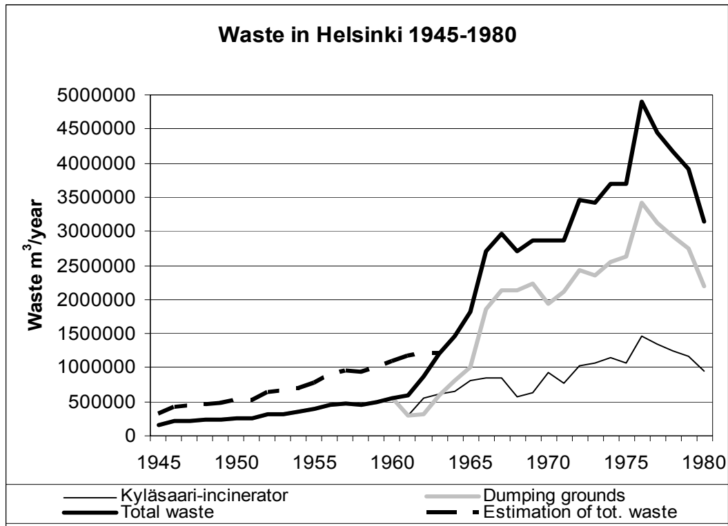
Figure 3: Total waste and the shares of waste disposed by tipping and incineration during 1945-1980. (BSP, Annual Yearbooks 1945-1980) (For the estimation of total waste: see Fig.1)
